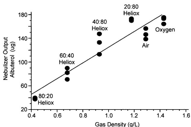
Fig. 4. The output of aerosol from an AeroTech II nebulizer (operated at the same driving-gas flow rate [6 L/min] with each gas mixture) is positively correlated with gas density.  $Y = -7.849 + 132.715X$ ,  $r^2 = 0.891$ ,  $r = 0.944$ ,  $p < 0.001$ . Heliox = helium-oxygen mixture (heliox ratio values [eg, 80:20] indicate percentages of helium and oxygen, respectively). (Adapted from Reference 12, with permission.)
