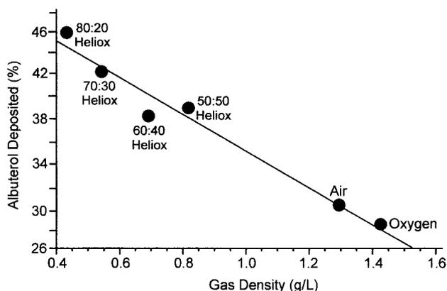
Fig. 6. Deposition of albuterol from a pressurized metered-dose inhaler increases as gas density decreases.  $Y = 51.667 - 16.77X$ ,  $r^2 = 0.965$ ,  $p < 0.005$ . Heliox = helium-oxygen mixture (heliox ratio values [eg, 80:20] indicate percentages of helium and oxygen, respectively). (Adapted from Reference 12, with permission.)
