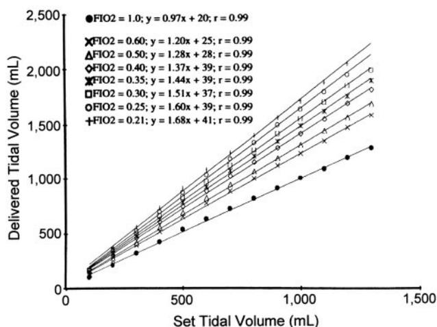
Fig. 8. Relationship between the tidal volume set on the ventilator and the tidal volume actually delivered by the ventilator, at various fractions of inspired oxygen (F<sub>IO<sub>2</sub></sub>), with corresponding regression equations, for 3 ventilators: Veolar FT, Galileo, and Evita 2. (Adapted from Reference 9.)
