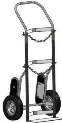
Part No. 1182 Model: 8001 Dim: 43.5"Hx20"Wx16.5"D Zinc Plated
